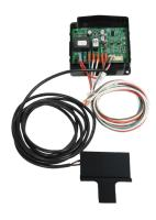
**Standard mitigation control kit (S)** – turns on indoor blower to dissipate refrigerant concentration and cuts power to outdoor unit to stop new refrigerant from entering the space. Kit includes all components needed for RDS installation.
